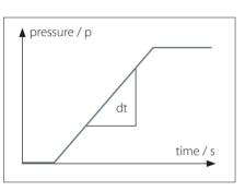
The maximum pressure change rate for mechanical pressure switches is 1,000 bar/s. For SUCO electronic pressure monitoring products the maximum pressure change rate can be up to 5,000 bar/s.
