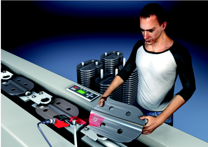
Figure 3.3: Application example: reading 2D-codes in presentation mode
