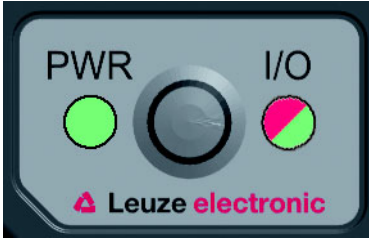
Figure 6.1: LEDs of the LSIS 22x
